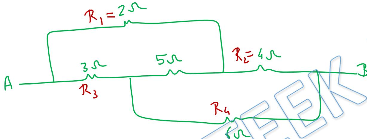
$$\text{Since } \frac{R_1}{R_2} = \frac{R_3}{R_4} = \frac{1}{2} \Rightarrow \text{bridge is balanced}$$
