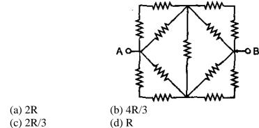
Q 8. Eight resistances each of resistance  $50\Omega$  are connected in the circuit as shown in figure. The equivalent resistance between A and B is:
